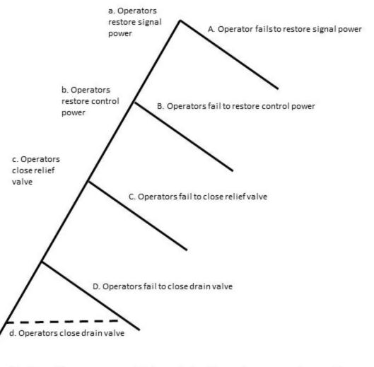
Note: Pressure relief and drain valves are in series – closing either valve gives desired outcome
